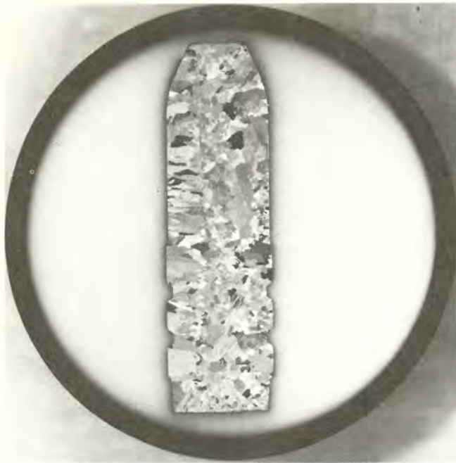
Figure 5. (2.7X) Macrograph of a soft lead bullet (Lee C309-190F) sectioned to half diameter and polished. The grain sizes and shapes are representative of those found in alloyed bullets although alloying generally produces a more uniform grain size.
