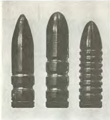
Fig. 13: The 3 basic forms of cast bullets: (l. to r.) No. 311334, short body and long bore-riding forward part; No. 311284, body and forward part both of good length; and No. 311467, long body and very little forward part
