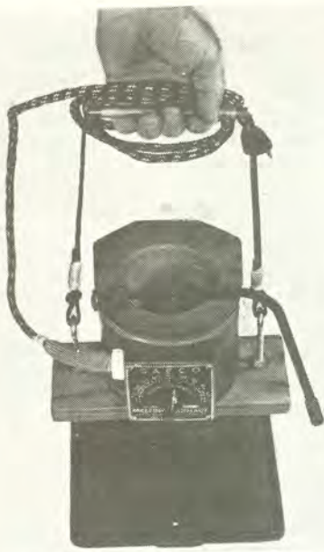
Fig. 9: Carrying lead pot outdoors for fluxing can be done with a suitable sling. This one is based on a strip of \frac{3}{4} " plywood, 3\frac{1}{2} " wide. A hole at its midpoint fits over the spout on bottom of pot, preventing slipping. The long eyebolts bring the points of attachment of the bail above the pot's center of gravity, so it is stable when carried
