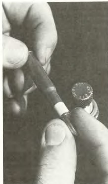
Case necks should be expanded slightly larger than bullet diameter to 1/8" depth to permit hand starting of patched bullet.
