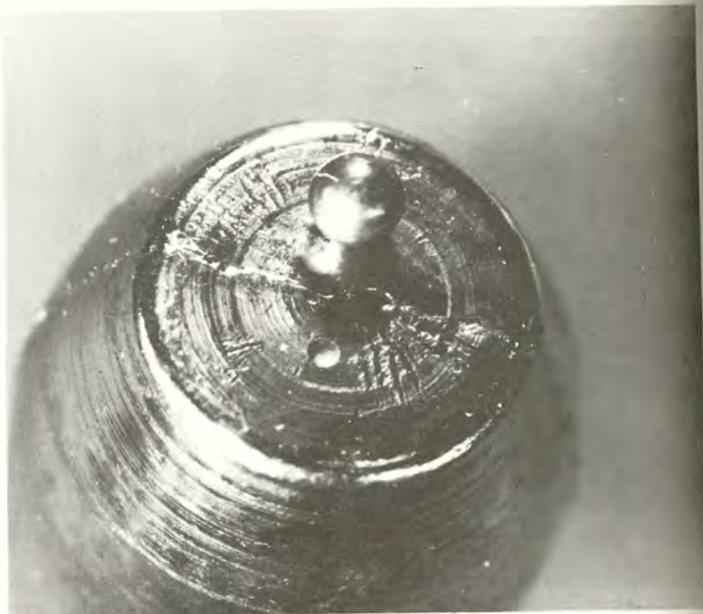
(12X) The stainless steel ball used for hardness testing, shown here on the nose of a Lee C309-170F bullet. The indentation shown is 0.39 mm. in diameter and with the 4 kg. load corresponds to a Meyer hardness of 33.5.
