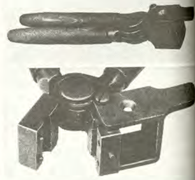
Pope cal. .33 point-cutoff bullet mold shown closed (top) and open.
