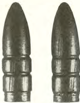
Fig. 3: The mechanism of cast-bullet success and failure. Left-hand bullet was fired with 10 grs. Unique. It passed through the rifle bore truly point-forward and concentric. (These bullets were fired with gas checks, which came off in the recovery medium.) Right-hand bullet was fired with 18 grs. Unique. While there is no sign of rifling failure, and the load is quite safe, the bullet is badly cocked by the force of the powder gas applied to it. A bullet in this condition is unbalanced and also will yaw badly on leaving the bore, resulting in wild shooting. Completely successful cast-bullet ammunition can be loaded with any rifle powder whatever, but the charge must be comparatively light for the powder chosen. There are some other factors important to cast-bullet loading, but this is the critical one
