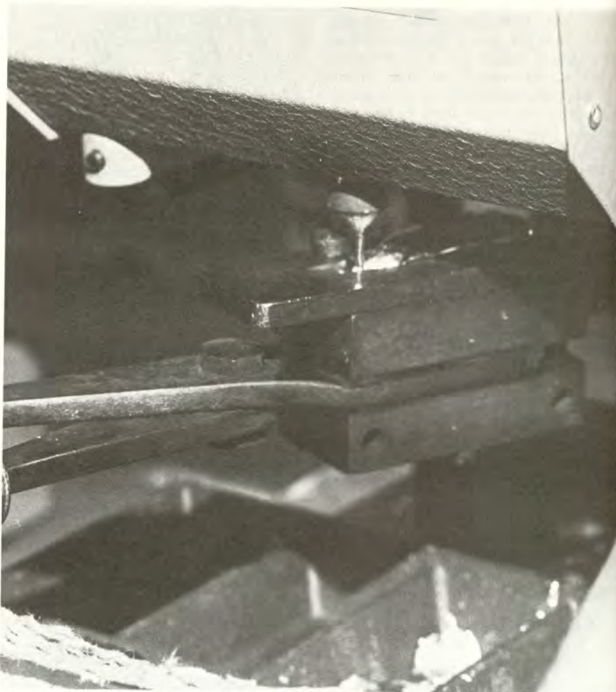
Four-cavity gang moulds make fast production easy. Hensley & Gibbs, Lyman, Saeco and NEI are popular suppliers of pistol gang moulds for target shooters. A bottom pour pot of large capacity is desirable to get best performance from multicavity moulds.
