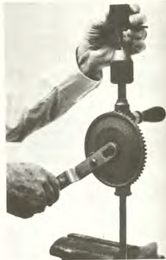
Cleaning bullet mold by slowly rotating brass brush in cavity (see text).
