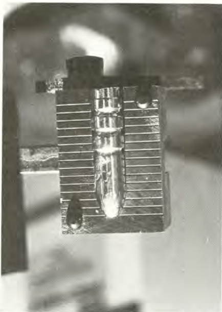
Too cool a casting temperature, or oil contamination of the mould, causes bullets to be wrinkled and not filled out.
