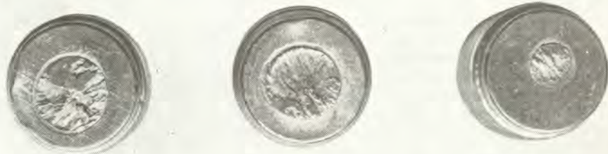
Various cut-off results in cast rifle bullets. (l. to r.) Large, rough cut-off from large dull-edged sprue hole, smoother cut-off from large sharp-edged hole, desirable bullet base produced by small sprue hole.
