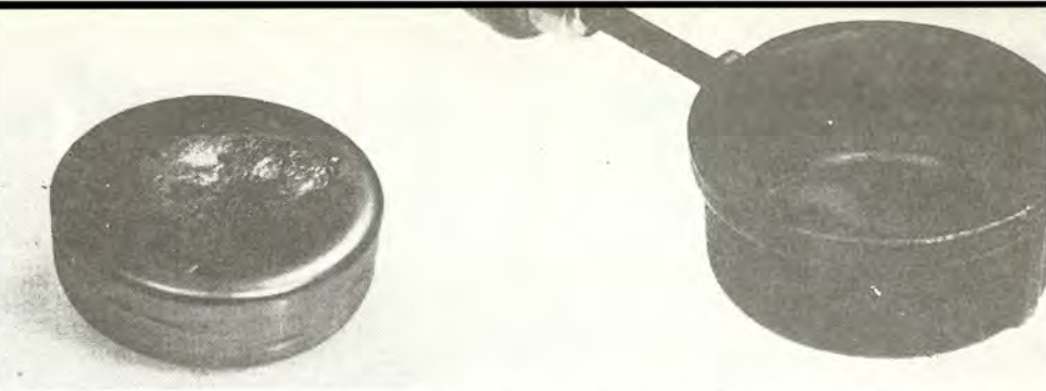
Fig. 2: Sample pieces can if desired be cast in shape offering large work surface. Mold is iron pipe cap with threads bored out on slight taper. Bottom must be faced very smooth, to leave suitably smooth work surface on cast piece
