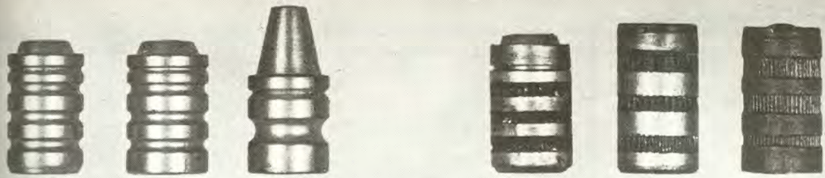
Bullets used in handloads in these tests. (l. to r.) H&G No. 50 BB, H&G No. 50, H&G No. 73, custom target wadcutter, custom hollow-base target wadcutter, Remington No. 22850 hollow-base target wadcutter.
