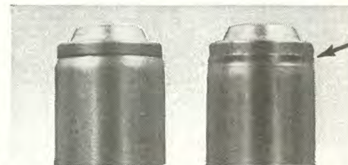
Specially formed heavy crimp (arrow, r.) was unsuccessful in improving grouping. Standard crimp shown for comparison.
