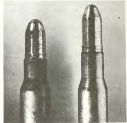
The effects of severe (left) and slight interference (right) of the forcing cone with cast bullets as described in text.
