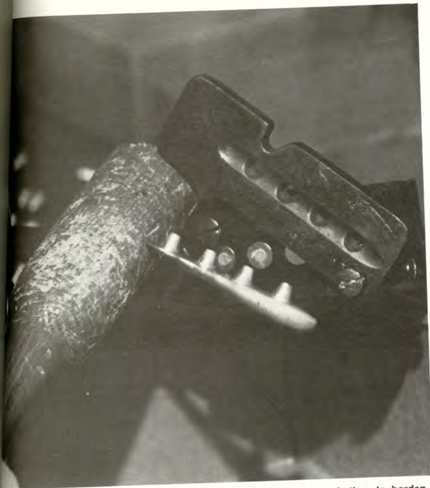
Knock off the sprue with a wooden mallet after giving it enough time to harden completely. Premature cutting of the sprue smears semi-molten metal across the blocks and damages bullet bases. Drop the sprue into a box for easy recovery and subsequent remelting.
