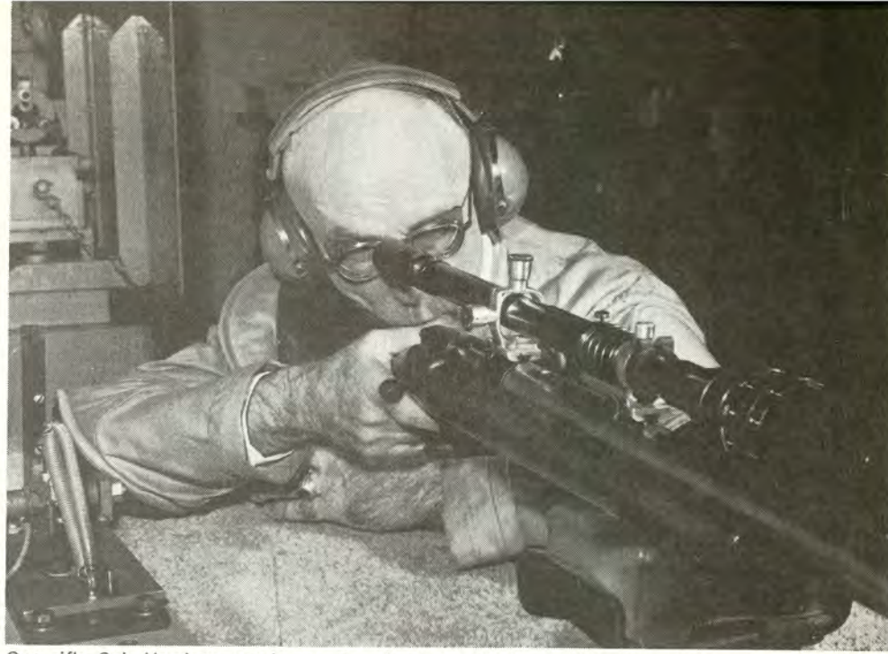
One rifle Col. Harrison used over the six-year period was this Rem .40X, cal. .308 Win., single-shot, bench model with Hart stainless heavy barrel rifled one turn in 12". Scope is a Unertl 15X Programmer-200 in Unertl Posa-mounts. Total wt. is 18 lbs. 1 oz.
