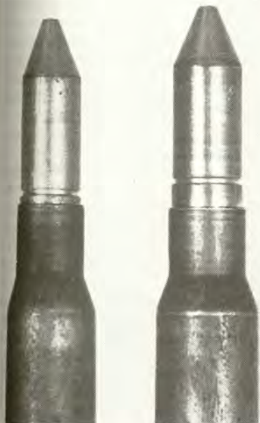
Diameter of bullet body affects seating depth. (l. to r.) Bullet of .3105" diameter as necessarily seated for use in a new .308 Winchester match barrel, and same bullet sized .3085" seated for use in same barrel.
