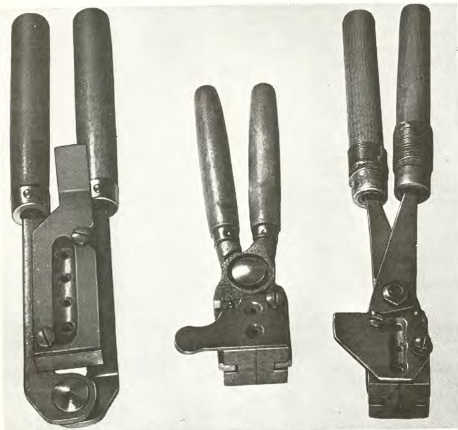
(l. to r.) Gang mold with channel sprue plate; multiple mold with individual-hole sprue plate; mold with individual-hole plate modified by milling and polishing channel between holes.
