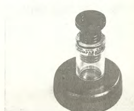
Fig. 5: Inexpensive pocket comparator is neat and convenient tool for same measurement, but does not give better results than micrometer caliper
