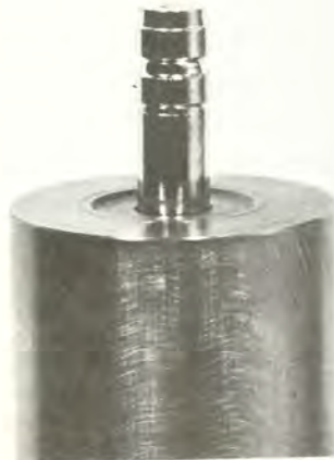
Cylindrical part of a cast bullet must not enter the rifle muzzle. This simple check for bore fit requires no measuring devices.
