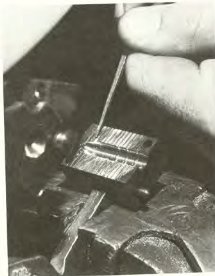
Best method to orient the bullet is to file a small index mark on the edge of the mould cavity, which leaves a small bump on the bullet, near the nose where it does least harm. This is indexed at 12:00 for each shot, and can be removed with the thumb-nail.
