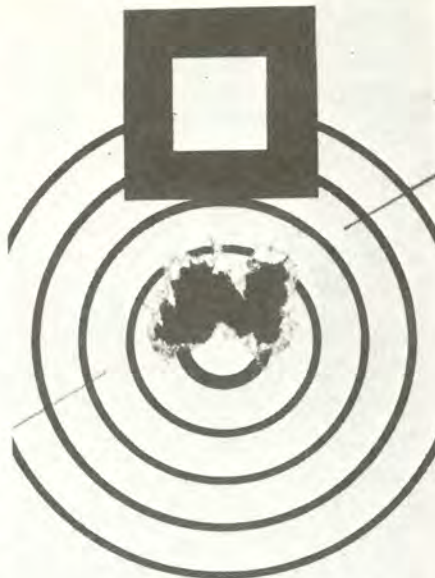
10-shot group at 100 yds. measures .580". Fired by the author Sept. 16, 1978 at the Cast Bullet Association National Matches.
