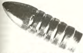
Defect caused by severe zinc contamination. Less contamination may show only frosting on bullet bands and grooves.
