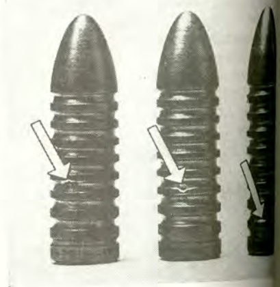
Fig. 10: Sizing does not remove most defects, since they are not limited to tops of the bullet bands. Sized bullets shown here have defects (see arrows) which are not removed by sizing but only made inconspicuous under a smoothed coat of grease. Out-of-roundness, being all over the bullet, is still less removed by sizing.
