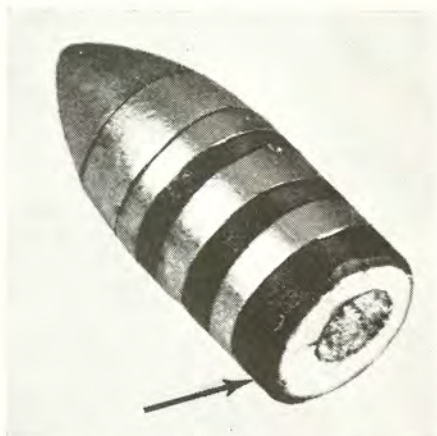
Gas-check bullet with gas check omitted and bullet lubricant on shank (arrow).
