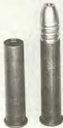
Reaming sized .45-70 case mouth to .460" diameter to a depth of about .11" allows hand starting of .459" diameter cast bullet.
