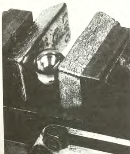
Measuring hardness of bullet metal sample by comparative indentation (see text).
