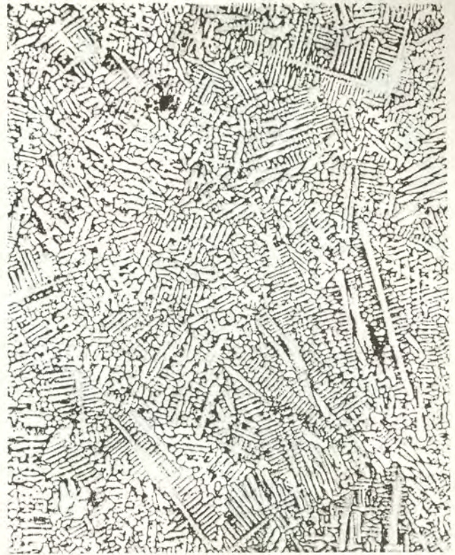
Figure 4. (100X) At this lower magnifications, this micrograph shows at least twelve "trees" in various orientations. The photograph was taken about 1/10" from base of a lead-5% antimony bullet. The small black spot near top of the picture is a shrinkage cavity formed when the eutectic material contracted on freezing.
