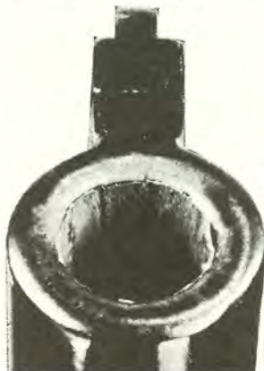
Heavy bore leading from prolonged firing of .357 Magnum factory ammunition
