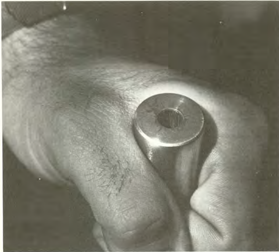
Leading destroys cast bullet accuracy. It can be caused by poor lubrication, gas cutting, soft alloy or too high velocity.
