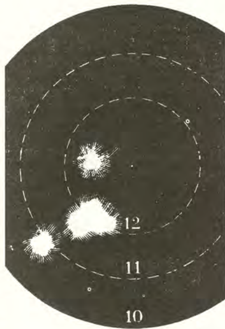
The target referred to, shown actual size. For verification, correct diameters of the 10, 11, and 12 rings are 3.36", 2.33" and 1.41".
