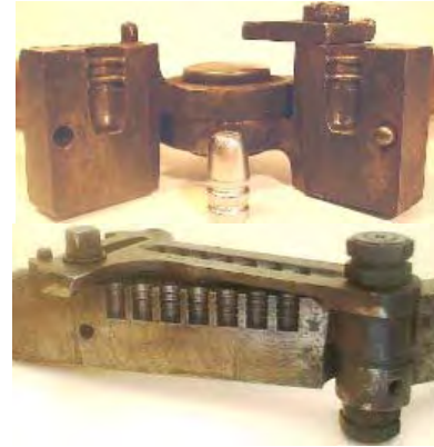
Examples of an early Ideal single-cavity mould (the 3118 for the .32-20) and multi-cavity Armory moulds (an Ideal 7-cavity mould for the 360344 wadcutter).
