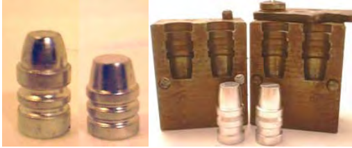
Early revolver bullet designs did not include a dedicated crimp groove (e.g. the Ideal 360271 and 360345 target bullets shown at left). Elmer Keith integrated a beveled crimp groove into the Ideal/Lyman 358429 (right) and most revolver bullets designed since then have followed suit.
