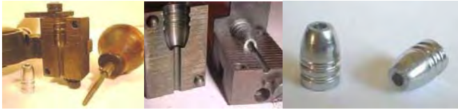
The first HP moulds suitable for use in handguns. These bullets were designed as "express bullets" for use in rifles, but also could be fired in revolvers (all were listed in the Ideal Handbook #9, circa 1897); the Ideal 31133 HP for the .32-20; Ideal 40090 HP for the .38-40, and the Ideal 42499 HP for the .44-40.
