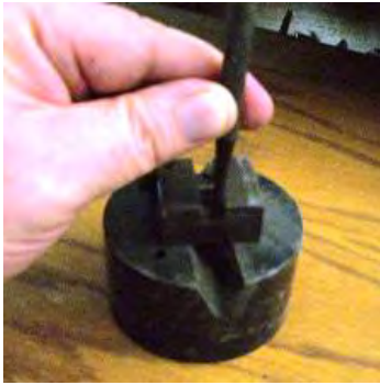
Picture showing how to properly tap out alignment pins. (Lyman Mould shown)
