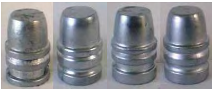
Elmer Keith's original design for the .45 Colt was the Ideal 454424 (on the left, flat-bottomed grease groove). Later, Lyman modified Keith's design to include a rounded grease groove (on right). Later on, Lyman modified this design and re-numbered it as the 452424, which has also been produced in both a flat-bottomed grease groove and rounded grease groove.
