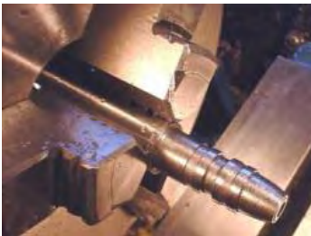
Turning the 410459 pilot (rough pilot profile)
