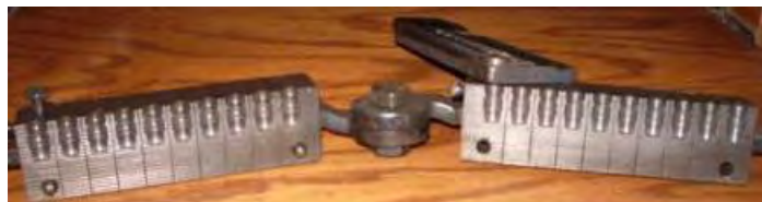
A well-used Hensley & Gibbs 10-cavity #51BB .38 semi-wadcutter mould (note the particularly massive sprue plate).
