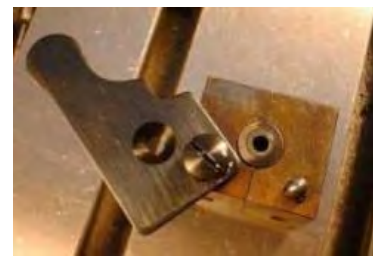
The finished pilot and Lyman 410459 mould; the pilot in place.
