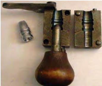
Shortly after designing the 429421, Elmer Keith followed up with a hollow-base version (Ideal 429422).
