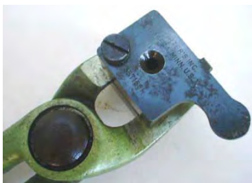
A single-cavity Herter's .38/.357 SWC mould mould cut by Lyman, with a 358156 cavity, with the Herter's sprue plate.
