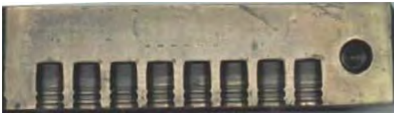
Frankfurt Arsenal gang mould for a bullet design similar to the ogival wadcutter or WFN profile
