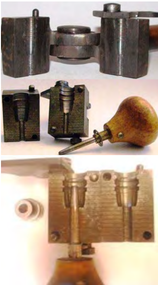
Ideal single-cavity 3118 mould for the .32-20 (integral handles).
