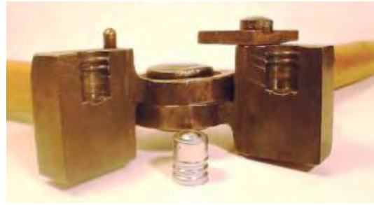
Note the lack of alignment pins and the hand-cut vent lines.
