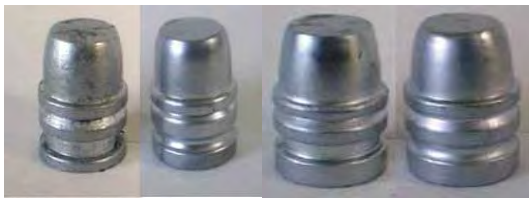
The original Ideal 454424 (left, with "square-cut" grease groove) alongside the later Lyman 454424 with a rounded grease groove. Later Lyman would re-number this to 452424, and at different times has offered that design with both flat and round grease grooves (right hand photo).
