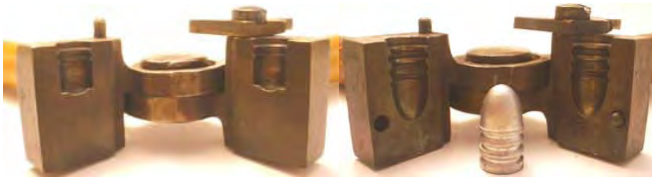
Early moulds relied on the hinge to align the mould blocks (e.g. this early Ideal .38 wadcutter mould). Later on alignment pins were added (e.g. Ideal 429251).
