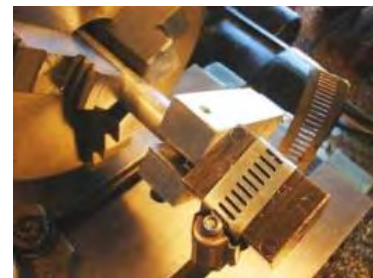
452460 mould clamped onto mandrel and held in place with dog.
