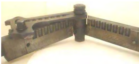
An Ideal Armory mould for the 360344 wadcutter.
