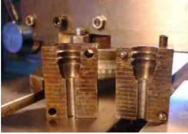
452460 with the block drilled
