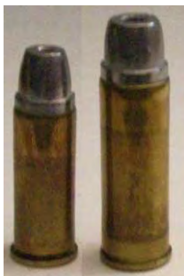
Keith designed the 429421 HP and 454424 HP for the .44 Special and .45 Colt (respectively).
