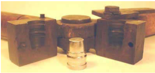
A copy of the Ideal 452423, made by Yankee Specialty Co. with integral handles (Yankee Specialty also made a few moulds with interchangeable blocks). This Depression-era mould is made from bronze, not iron.
