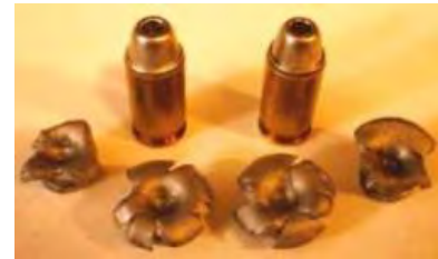
Fired with a muzzle velocity of 1100 fps, the 452460 HP demonstrated positive expansion in ballistic gelatin (bullets were cast of WW alloy)
