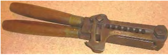
Ideal Armory moulds were multiple cavity gang-moulds (5, 6, 7-cavities, etc.). Rugged moulds for high production casting.
