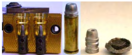
The beautiful work of Miha Prevac (45-270-SAA HP mould) makes bullets that shoot and expand very well indeed.
