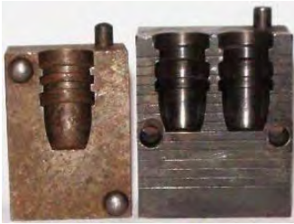
The Heath target bullet (Ideal 429336, left) compared to the Keith SWC (Ideal 429421, right).
