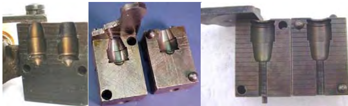
Examples of the Harvey Prot-X Bore cast bullet designs (e.g. the .38 and .45 Harvey moulds shown). Some of the Harvey designs were even available in HP form (e.g. the .44 HP mould shown).
