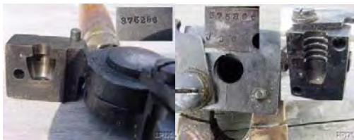
An example of a 2-part bullet (Ideal 375296). The small mushroom-shaped tip would be cast out of a soft alloy (like pure lead), then that piece would be inserted into the regular cavity of the bullet mould and the remainder of the bullet would be cast of somewhat harder alloy.
