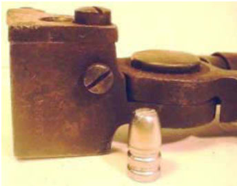
Ideal single-cavity 3118 mould for the .32-20 (integral handles).
