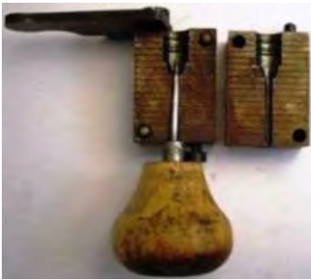
Occasionally one runs across some rather odd-ball HP moulds, in this case the Lyman 313445 HP.
