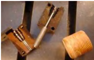
Mould blocks after HP channel has been drilled out, and the roughed out HP pin and knob.
