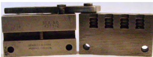
An example of a Type I wadcutter (H&G #280, .32 caliber wadcutter). Note the lack of "button-nose" and no crimp groove.
