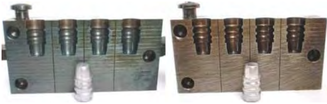
The Lyman 358156 GC-SWC (designed by Ray Thompson in the early 1950s), and its plain-based progenitor, the 357446 ("the Standard Bullet for the .357 Magnum") shown for comparison.
