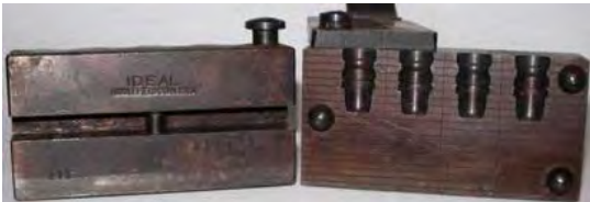
An example of a 4-cavity Ideal mould (Ideal 358477).
