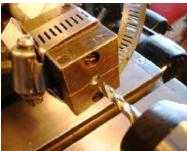
Taking the plunge cut with an end-mill to cut the HP pin channel.
