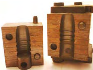
An example of a nose-pour mould (Hoch .41 caliber 210 grain mould).
