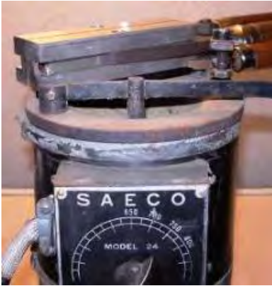
Picture showing heating an aluminum mould sprue plate down.
