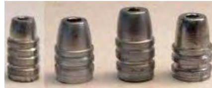
The hollow-points of Ray Thompson (l-r: Lyman 358156 HP, 429215 HP, 429244 HP and 452491 HP).
