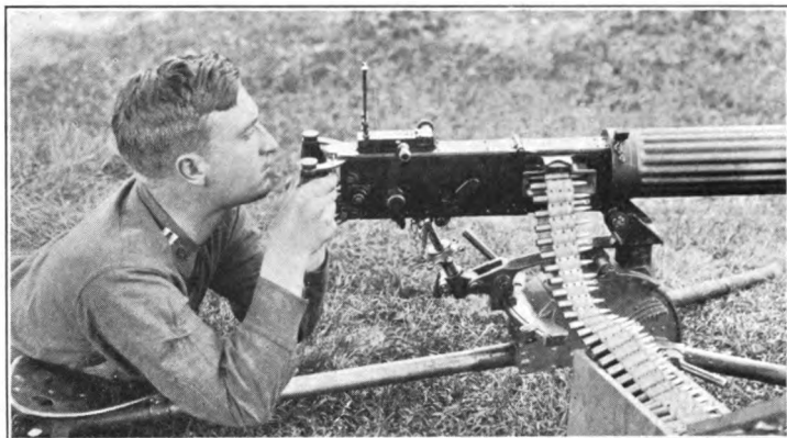
Vickers gun, second position stoppage
