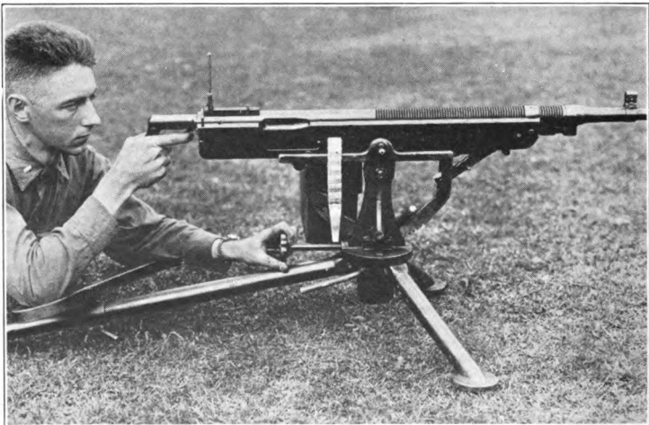
Third characteristic position of gas lever. Note that gas lever is all the way back.
