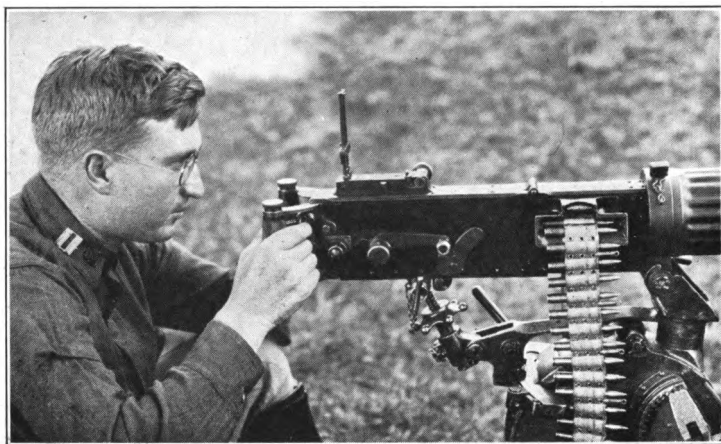
Third position stoppage. Note that roller handle lacks half an inch of being onto roller
