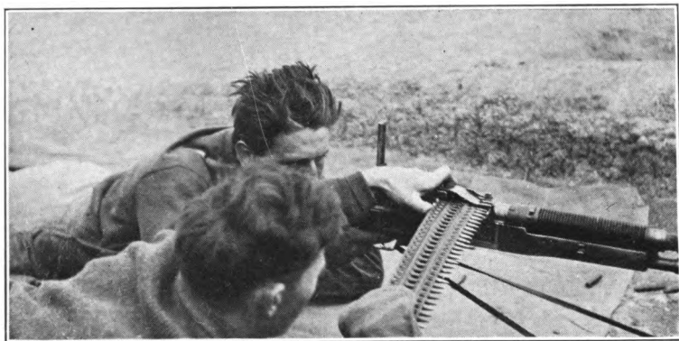
The proper method of loading. Note that outer end of strip is pressed down to prevent front end of strip from getting under feed guide.
