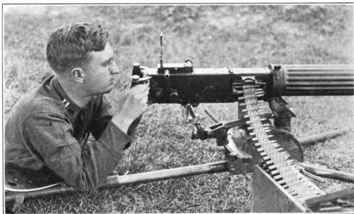
Vickers gun, first position stoppage
