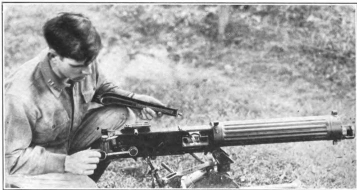
Testing friction of recoiling parts. Note position of roller handle, also that recoil spring is removed during this test.
