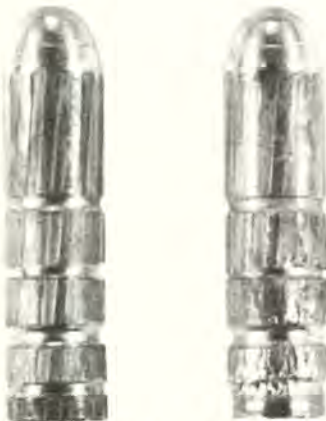
Deep seated bullet shows gas cutting and shed its gas-check. Correctly seated bullet retained gas-check without gas cutting.
