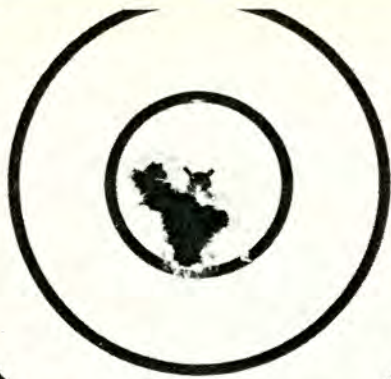
Five-shot group at 100 yds. measures .49" between centers. Target shown actual size. The first 5 100-yd. groups averaged .766".
