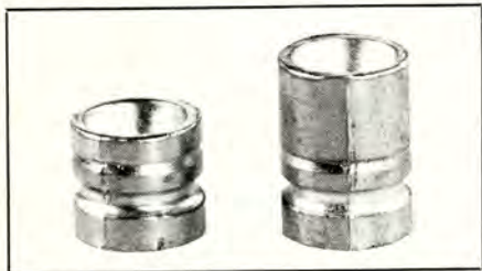
Lyman #452626 composite jacket (l.) with 232-gr. cup-point wadcutter produced in same mould, after a simple modification.
