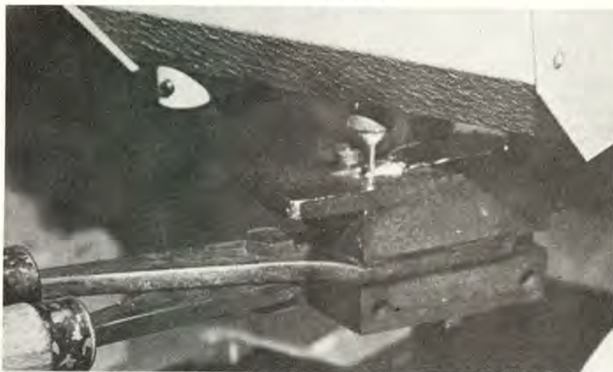
Shooters unwilling to exercise the time and effort needed to cast and select good bullets should rely on factory swaged or jacketed ones instead, but the patient, careful caster can do well with a bottom-pour pot and 4-cavity mould, making suitable bullets for most practice and competition.
