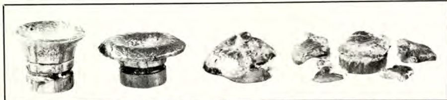
#452626 cup-point bullets cast from 50-50 wheelweights and plumber's lead, and shot from M1917 S&W .45 Auto Rim (left to right) at 689 f.p.s., 767 f.p.s., 876 f.p.s. and 921 f.p.s. Use softer lead below 700 f.p.s., and limit velocity to about 900 f.p.s. in any case.
