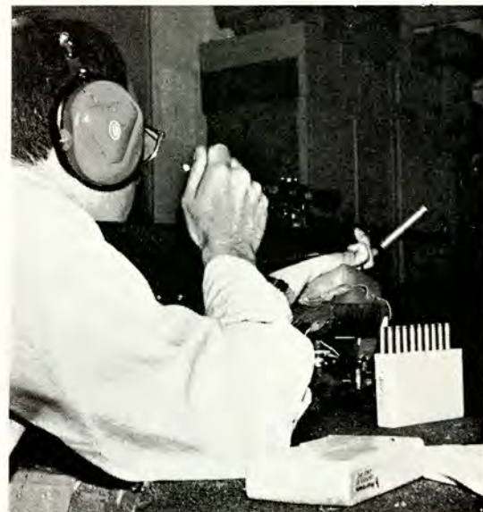
Several hundred rounds were fired in testing, but field experience emphasized need for secure crimping of bullets for hunting.
