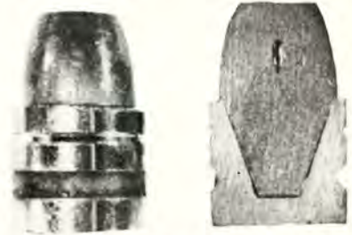
Sectioned #452636 .45 Colt composite shows its two-piece construction. #358624 and #429625 are made for .357 Mag. and .44 Mag.
