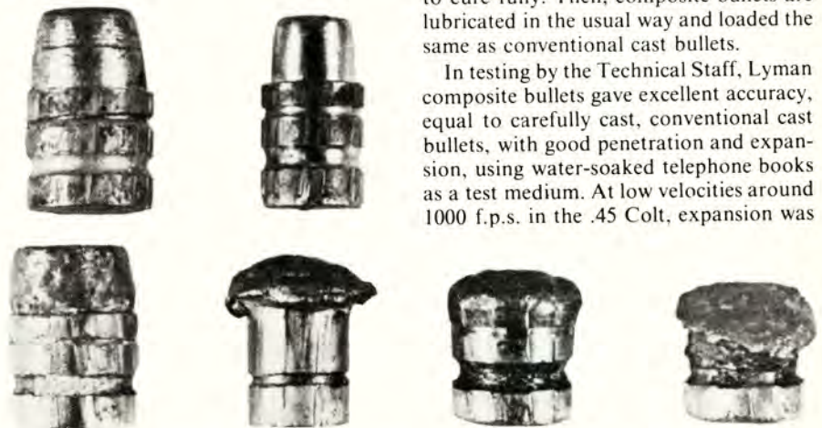
Wheelweight-metal Keith bullets don't expand. (Top): #454424 shot into wet paper at 1089 f.p.s. and #358477 at 1317 f.p.s. Composites expanded (bottom): #452636 at 1002 f.p.s., #358624 at 1247 f.p.s., #429625 at 1518 f.p.s., and #429625 at 1600 f.p.s. from T/C Contender pistol.
