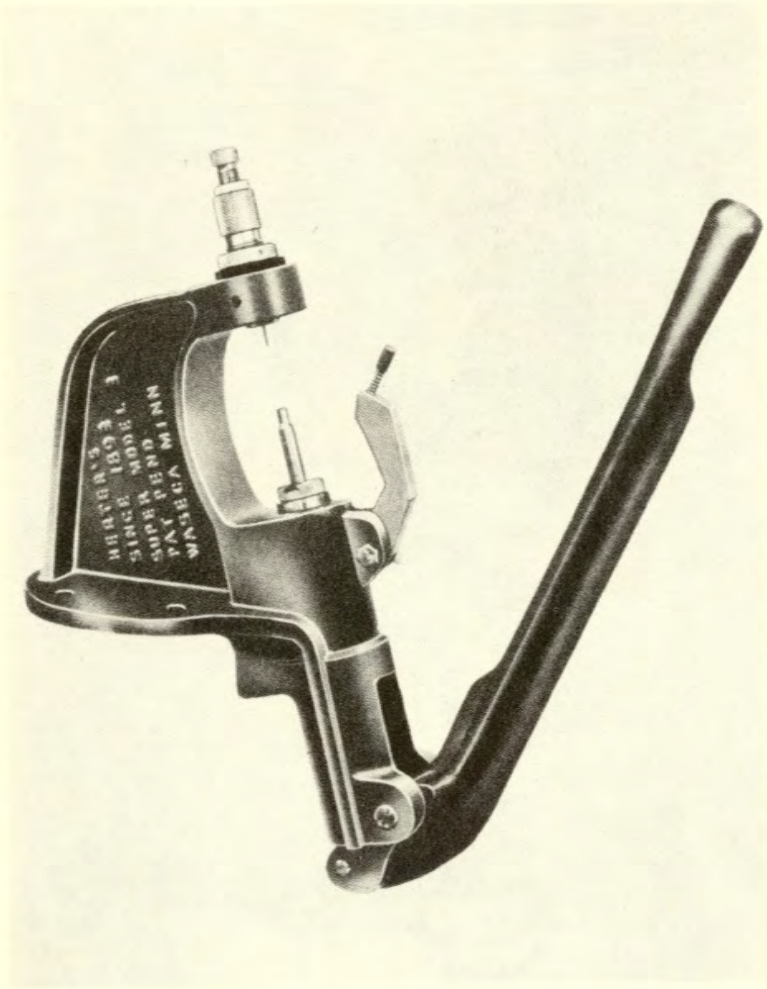
Herter's Model 3 Loading Press is the least expensive of all heavy bench presses, and an excellent one too. It operates on the down stroke of the lever, and case holders can be interchanged in a few seconds. Uses \frac{7}{8} " X 14 dies.
