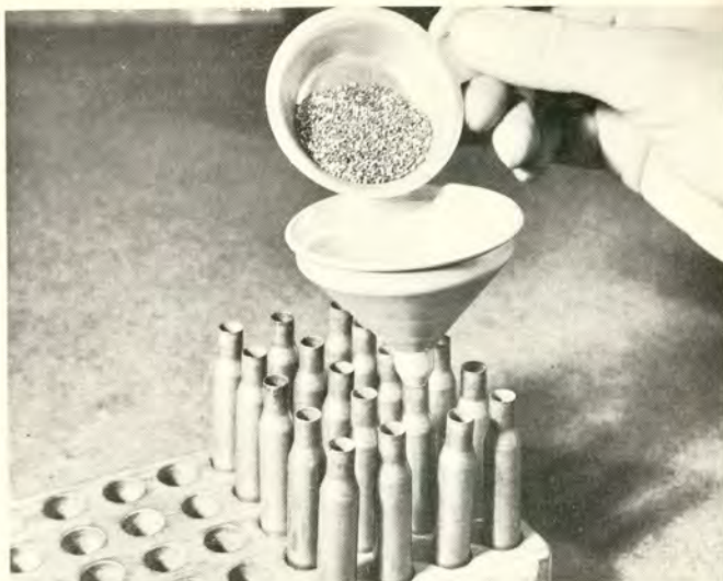
Loading powder. This operation should only be done when full attention can be given to it. Visually check all cases to make sure each has the correct amount of powder before seating bullets, or use a depth gauge, easily made.
