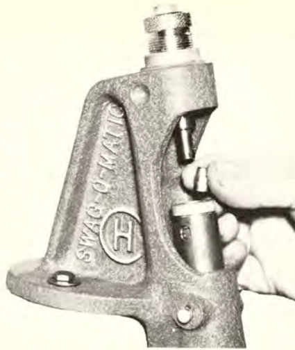
C-H Swag-O-Matic operates like a short stroke reloading press to make perfect bullets. This is the market's hottest item.
