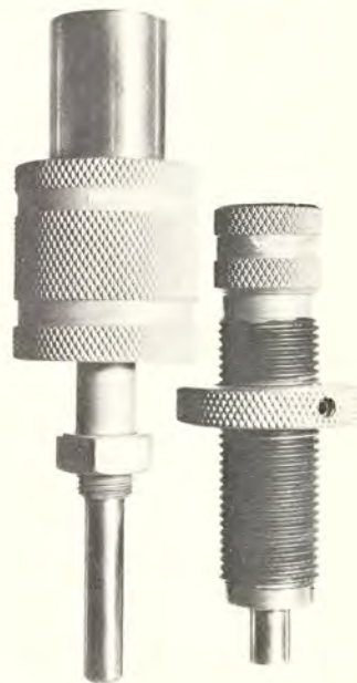
Hollywood Gun Shop swaging dies, ultra precisely made, were developed by Lyle Corcoran in 1954.
