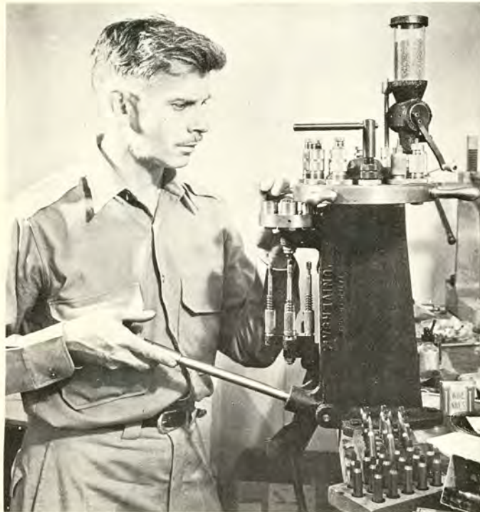
Many elaborate tools are used by some handloaders. Here the author is using the Universal multiple turret tool with a variety of dies in different calibers in the head. Note the shell holder turret set up with four types, and the priming rod turret with rods for small and large primers, both round and flat face.
