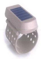
The device is ~35g, and as seen above, is fitted to a collar on the lower neck of the geese. If found on a dead bird, cutting through the neck collar is the easiest solution to removing them without damaging the device.
